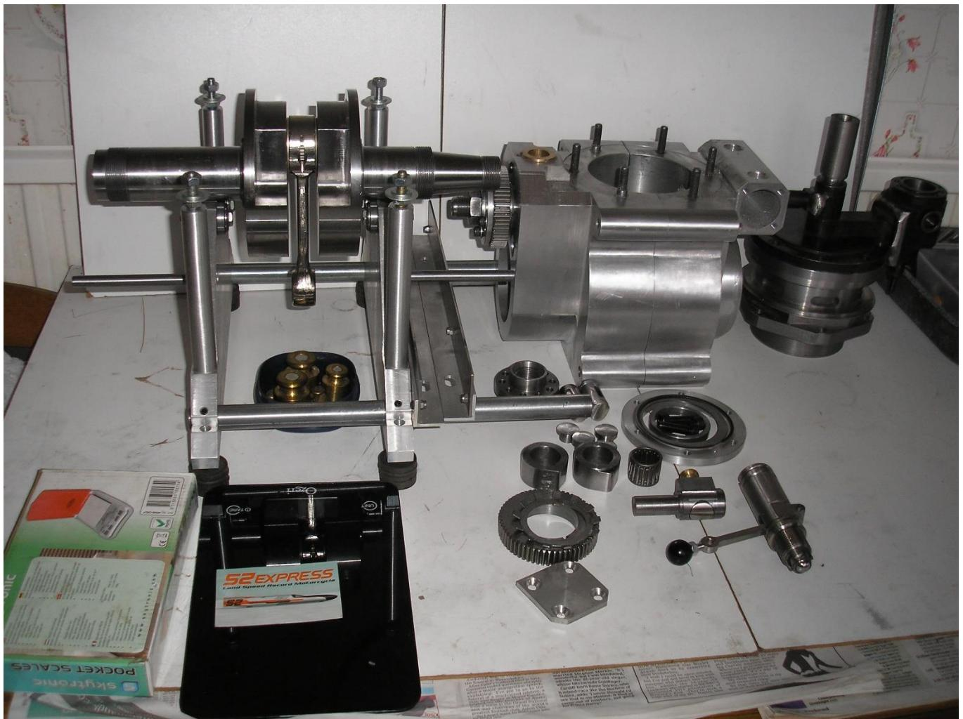
At the moment in the workshop, Paul is performing some weight reduction on the piston before working out the balance factor for the crankshaft.
